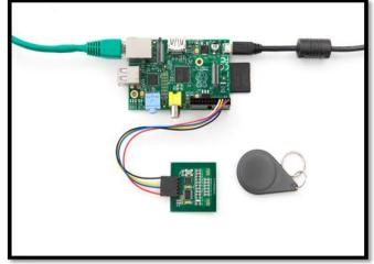
Fig. 2 RFID and Raspberry Pi Interface
